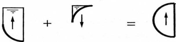
$$F_V = \gamma V = 9/806 \times (2) \times \left( \frac{\pi \times 2^2}{4} \times 8 \right) = 492/v kN$$
